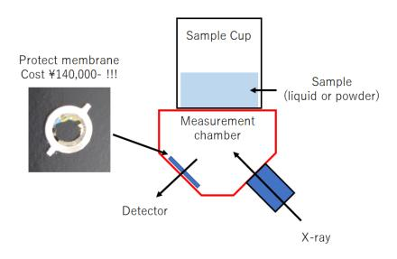
If the sample falls into the chamber, the machine got error and the protect membrane may be damaged. So, please endure the following.
